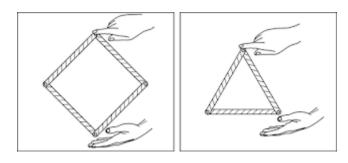
No, the triangle is not distorted but the quadrilateral is distorted.
