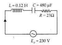
(a) At resonant frequency, the current amplitude is maximum.
