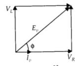
Phase lag,  $\tan \phi = \frac{X_L}{R} = 1.57$  $\phi = \tan^{-1}(1.57) = 57.5^\circ$  or  $\phi = 0.32 \pi$  radian Time lag,  $t = \phi/\omega = 3.2$  ms
