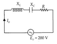
Average power transferred to the circuit in one complete cycle at resonance
