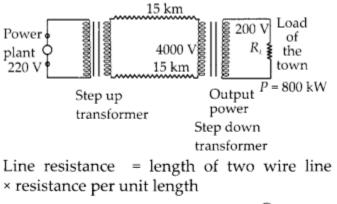
Line resistance (*R*) = 2 × 15 km × 0.5  $\frac{\Omega}{\text{km}}$  = 15  $\Omega$
