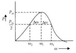
Now,  $\omega_1 - \omega_2 = R/L$  $[\omega_r + \Delta \omega] - [\omega_r - \Delta \omega] = R/L$  or  $\Delta \omega = R/L$
