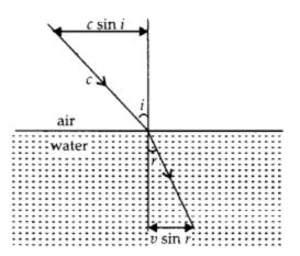
Considering a ray of light going from a rarer medium (air) to a denser medium (water). Let c = speed of light in vacuum (or air), v = speed of light in water, i = angle of incidence, and r = angle of refraction Then according to Newton's corpuscular theory,
