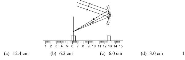
The focal length of the concave mirror in the following experimental set up is
