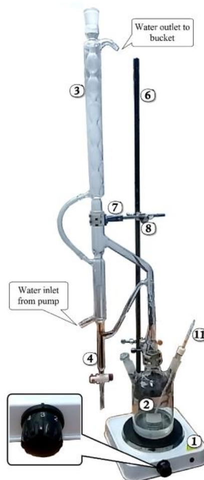
Figure 1. Hydrodistillation Apparatus, will be used to isolate nutmeg oil from nutmeg seeds
