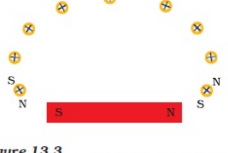
Figure 13.3 Drawing a magnetic field line with the help of a compass needle
